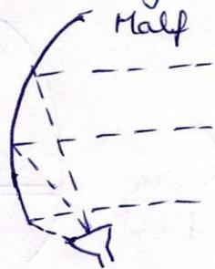
offset feed using waveguide horn
