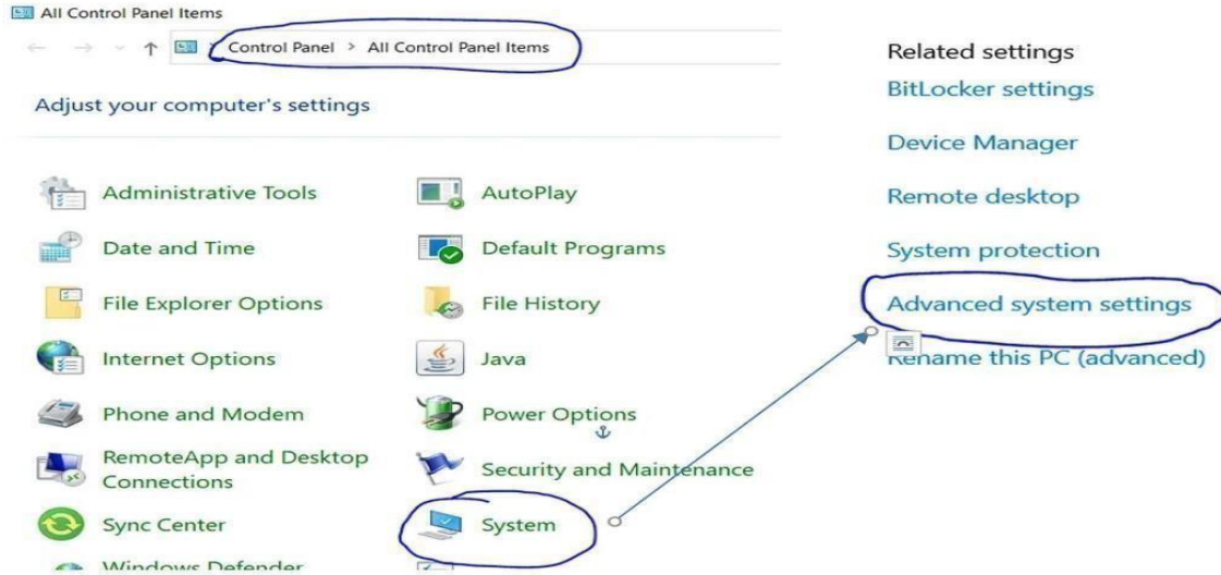
Fig. 5:- Path for Environment Variable.
