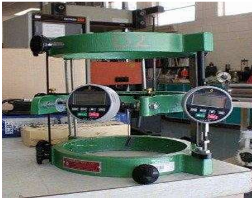
Fig: Setting up of Compressometer
